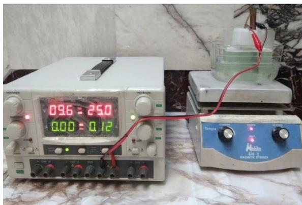
Figure 1. Electrochemical apparatus used to prepare the CuO/TiO<sub>2</sub> nanocomposites
