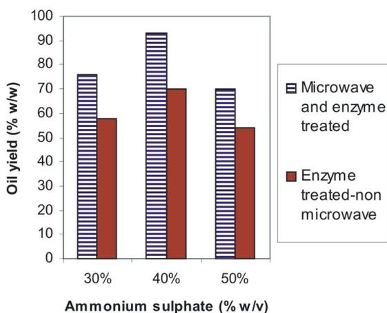
**Figure 3. Effect of varying amounts of ammonium sulphate in TPP on oil extraction at pH 7**
