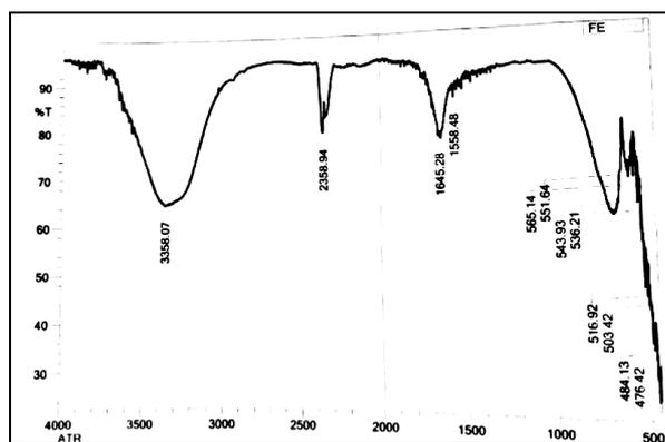
Figure 5. FTIR spectrum of Cu nanoparticles synthesized from Fenugreek seeds extract
