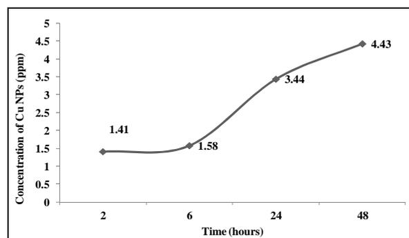
Figure 2. Cu NPs concentration at different time intervals with 15% seed extract added to 0.01M  $\text{CuSO}_4$  Solution
