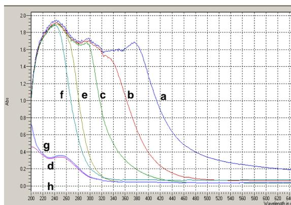
Figure 6. UV-Vis absorption spectrum of the DNA incubated with TiO<sub>2</sub> solution.
