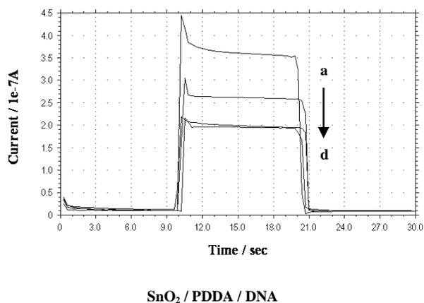
Figure 1. Anodic photocurrent response of Ru(bpy)<sub>2</sub>(dppz)<sup>2+</sup> bound to SnO<sub>2</sub> / PDDA / ds- DNA electrode after the DNA film was exposed to a: 2 mg mL<sup>-1</sup> psnp, b: 1 mg mL<sup>-1</sup> psnp, c: 0.5 mg mL<sup>-1</sup> psnp and d: phosphate buffer.
