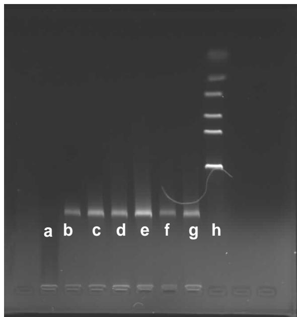
Figure 4. Agarose gel electrophoresis of the DNA incubated with TiO<sub>2</sub>
