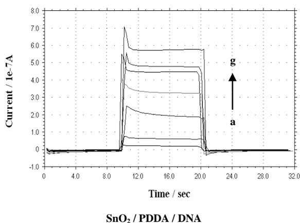
**Figure 2.** Anodic photocurrent response of Ru(bpy)<sub>2</sub>(dppz)<sup>2+</sup> bound to SnO<sub>2</sub> / PDDA / ds-DNA electrode after the DNA film was exposed to a: 1 mg mL<sup>-1</sup> of TiO<sub>2</sub>, b: 0.5 mg mL<sup>-1</sup> of TiO<sub>2</sub>, c: 0.1 mg mL<sup>-1</sup> of TiO<sub>2</sub>, d: 100μM Na<sub>2</sub>CO<sub>3</sub>, e: 50μM Na<sub>2</sub>CO<sub>3</sub>+2.5M H<sub>2</sub>O<sub>2</sub> f: 5 M H<sub>2</sub>O<sub>2</sub> and g: 20 mM sodium phosphate buffer (pH 7.3).
