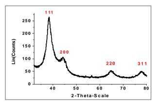
Figure 4. X-Ray diffraction (XRD) pattern showing Gel-AuNPs.
