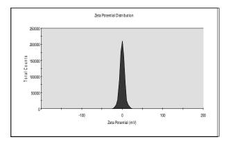
$\label{eq:figure 5.} \textbf{ Zeta potential spectrum of gelatin capped gold nano particles.}$
