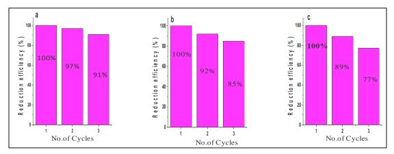
Figure 8. Percent reduction potential of glass supported Ge-AuNps recovered and re-used for 3 successive cycles (a) EB(b) MB (c) RB.
