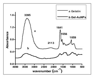
Figure 3. FTIR showing (a) pure gelatin (b) gelatin capped gold nanoparticles.
