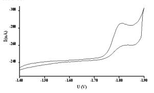
Figure 3. Cyclic voltammogram of 130  $\mu M$  DBP in 0.1M TBAB at HMDE at scan rate 100 mVs  $^{1}.$
