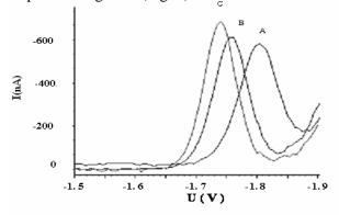
Figure 1. DP polarograms of 1.3 x  $10^4M$  DBP in the presence of 0.01 M of A) TEAI B) TBAB and C) TMAB.
