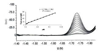
Figure 5. DPP calibration curve for aliphatic phthalates in the range of a) 0.3–160  $\mu$ M; b) 0.3–9  $\mu$ M. (insets show respective linear plots).
